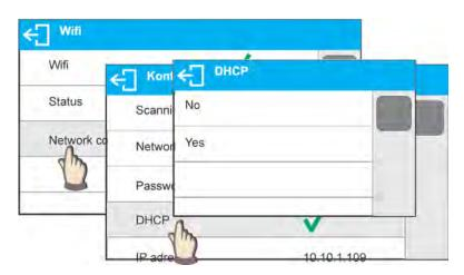
with DHCP set to NO value, enter manually IP; MASK; DEFAULT GATE parameters, with DHCP set to YES value, the balance software automatically reads and displays data assigned by Wi-Fi router by means of which the balance is to be connected,
