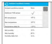
Ambient conditions module – parameter specifying module's working mode. Available options: None – readout of ambient condition module indications turned off; Record and alert – readout and record of indications into database turned on, option of display of warnings informing on ambient conditions change turned on, the warnings are displayed in accordance with the following tolerance values settings.
