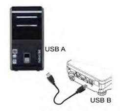
Having completed driver installation, connect balance to a computer, use 1,8meter long USB A/B cable maximally (in of already case connected balance, it is necessary to disconnect it and using USB cable connect the balance again).
