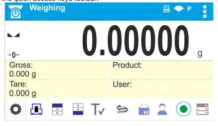
The system monitors balance level state. In case of level deviation, position of level marker is displayed on the screen ( correct levelling, incorrect levelling) and/or respective alarm is activated. Balance level setting proceeds.
