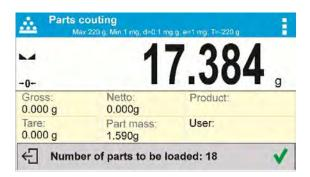
• The software automatically recalculates single part mass, next it moves to <Parts counting> mode displaying number of parts loaded on the weighing pan (pcs marking).
