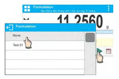
home screen is displayed, container weight is tared automatically, navigation bar with messages for ease of operation is shown,
