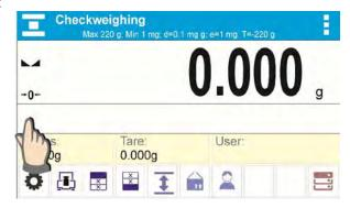
Press and hold for a while the spot where bar graph is to be placed.
