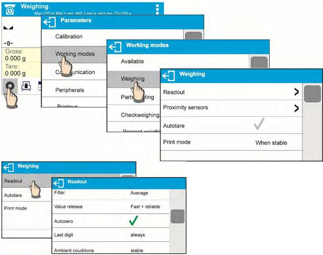
Filter level setting (function unavailable for the following profiles: Fast, Fast dosing, Precision)
