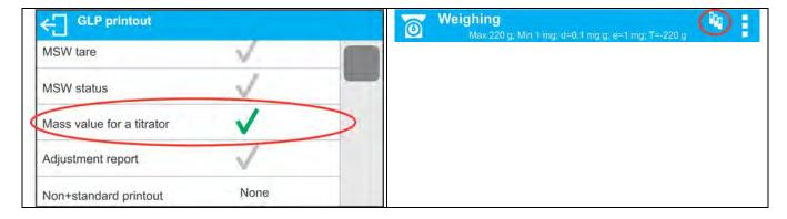
With <Yes> value on, a respective pictogram is displayed in the top bar of a home screen. The pictogram informs on special format of mass printout, tolerable by TITRATORS.
