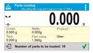
Put specified number of pieces on the weighing pan, when the result is stable (► stability pictogram displayed) press key to confirm,
