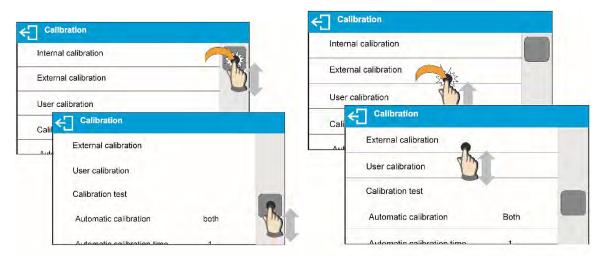
There are two methods for scrolling the screen of parameters window. The first one requires pressing, holding down and scrolling up or down the scrollbar located on the left. The second one requires pressing, holding down and scrolling up or down any point of the displayed window.
