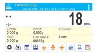
Stable measurement (stability pictogram displayed) can be printed, to do it press button.
