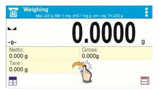
Press and hold for a while the spot where a given label is to be placed.
