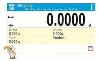
Press and hold for a while the spot where a given key is to be placed.
