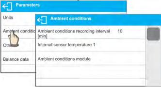
Ambient conditions recording interval [min]: parameter enabling you to specify record frequency
