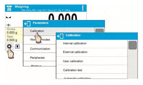
In order to enter balance menu, press <a></a> <PARAMETERS> button. Clicking any button comprised within information section, or clicking any button with particular parameter name, results with change of colour. This is for signalling purposes. If a given area has any function or action assigned, then it is performed automatically upon clicking (e.g. adjustment procedure), respectively a particular window with parameters or list of appropriate settings is displayed.
