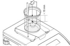
10. Upon confirmation of the second indication, the software automatically calculates measured liquid density, which is next displayed together with a respective message, report on measurement is sent to a selected printer port.
