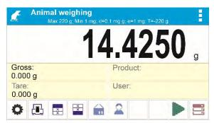
On completed mass determination process, "freezed" weighing result is displayed, the mass is automatically printed using the printer.
