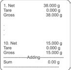
CAUTION: On adding process completion, only a summary is printed. The masses of particular samples are printed on confirmation.
