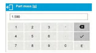
• Enter the requested value and confirm by pressing key, <Parts counting> mode is run with automatically specified part mass.
