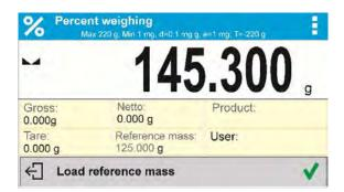
• 100.000% indication is displayed, loaded part weight is accepted as a reference mass, it is automatically recorded and displayed in reference mass field.
