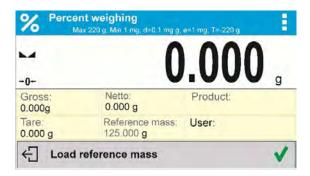
Load the part to be weighed and upon measurement stabilization press button for confirmation,
