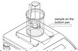
12. Upon confirmation of the second indication, the software automatically calculates measured solid density, which is next displayed together with a respective message, report on measurement is sent to a selected printer port.
