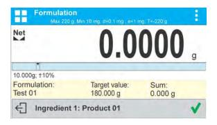
At the top of information area there is a bar graph, underneath the bar graph weight value that is to be dosed is displayed. Bar graph colour changes gradually depending on the ingredient weight (read Dosing section for detailed description of bar graph).
