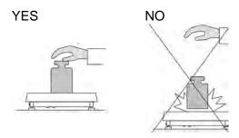
Place weighed loads centrally on the weighing pan:
