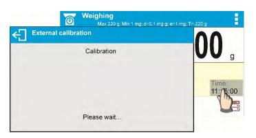
Press to develop an internal adjustment operation (internal adjustment function is assigned to the text field).
