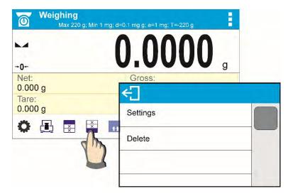
5. In order to rearrange widgets layout, it is necessary to delete already applied widgets first, and define new arrangement of buttons, labels and text fields next.
